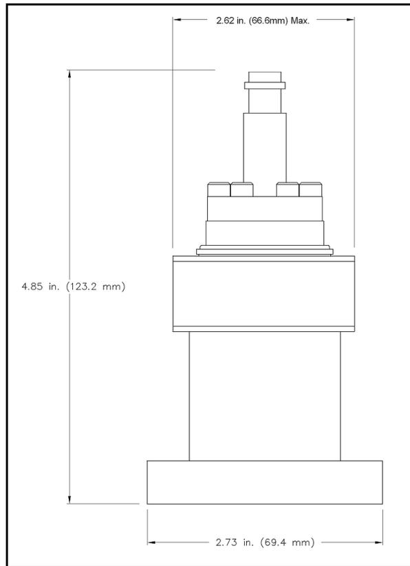
**Figure 1-1 Outline Drawing, IMG-300 Inverted Magnetron Gauge**
