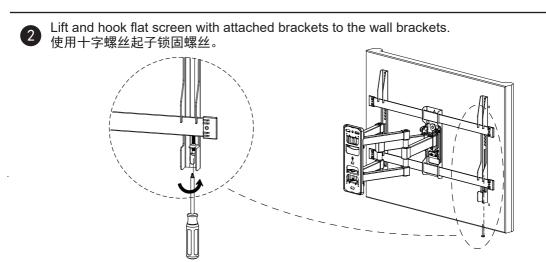
To adjust Tilt or Alignment of Flat Screen use open-end wrench and screw-driver. 若荧幕面板部份不平整,请使用开口扳手跟螺丝刀松开螺丝跟螺母,调整面板角度至水平后,再将螺丝跟螺母旋紧。
