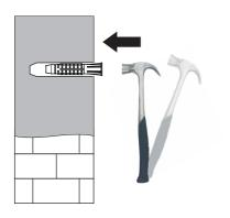
Secure the wall bracket using W-A Lag Bolt and W-C Washer 将墙板螺丝套上垫片,锁紧墙板。
