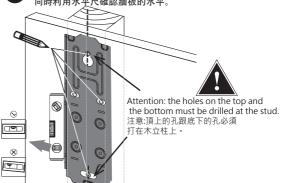
Secure one of W-A Lag Bolt and W-C Washer into the top pilot holes(x). Leave 0.6" (1.5 cm) visible. 將一個牆板螺絲套上墊片,鎖入最上面的牆孔,預留 0.6" (1.5cm) 螺絲長度。
