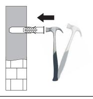
Secure one of W-A Lag Bolt and W-C Washer into the top pilot holes(x). Leave 0.6" (1.5 cm) visible. 將一個牆板螺絲套上墊片,鎖入最上面的牆孔,預留
