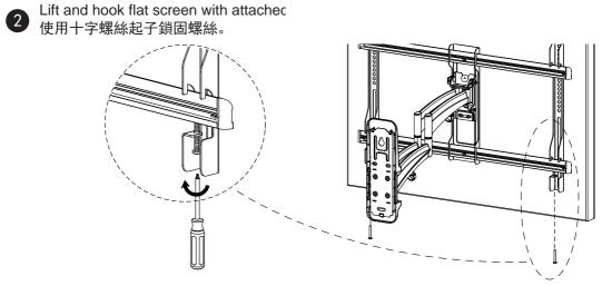
To adjust Tilt or Alignment of Flat Screen use open-end wrench and screw-driver. 若螢幕面板部份不平整,請使用開口扳手跟螺絲刀鬆開螺絲跟螺母,調整面板角度至水平後,再將螺絲跟螺母旋緊。
