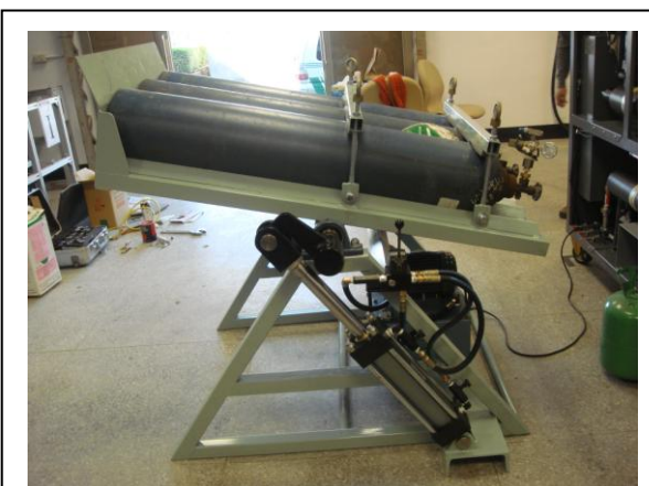
SF 6 Cylinders Moving Angle over 110 degree.
