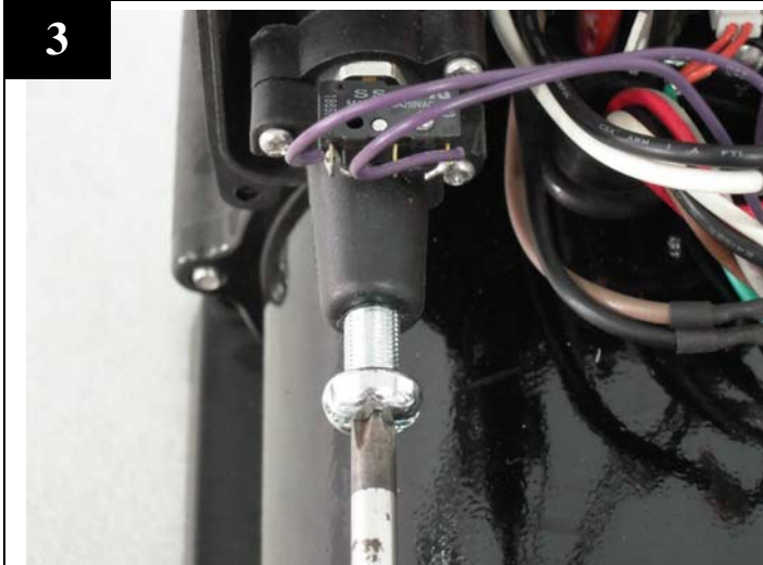
3 啟動電源且將壓力開關調整螺栓逆時針旋轉至最底
