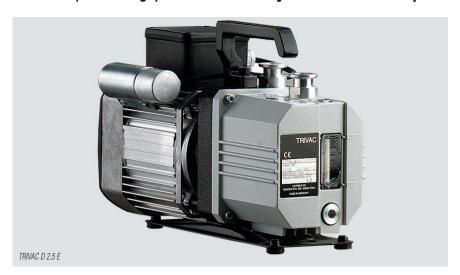
The TRIVAC E pump is an oil-sealed vacuum pump operating according to the rotary vane principle. Oil which is injected into the pump chamber is used for sealing, lubrication and cooling purposes.
